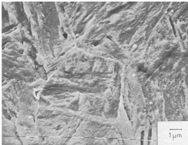
Figure 4 SEM picture of the martensitic microstructure of 1070 steel.
